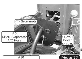
Firewall, **Engine Side** View
