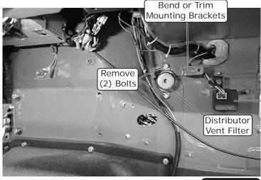
Remove and Relocate Relays
