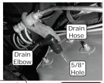
Firewall, Engine Side View
