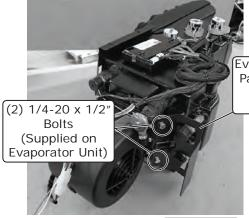
Evaporator Front Passenger Side Bracket 648264
